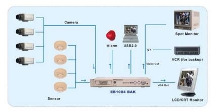
Connecting cameras, sensors, alarm, and display device
